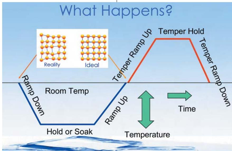
**Fig. 1 — Generalized cycle of cryogenic processing.**
